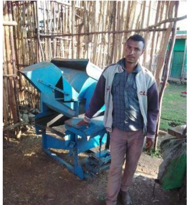
Nebo Obse Kimo with his mechanical thresher. Mr. Kimo threshes barley and wheat for 90 ETB per quintal. During busy periods (December to February), he serves an average of 10 customers and processes a total of 40 quintals per day. Mr. Kimo also sells wheat and pearled barley grains directly to consumers.
