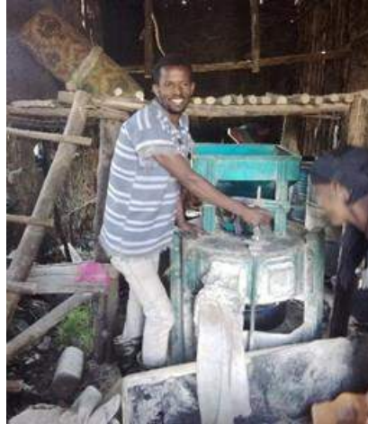
Abeyot Ayenew Asres with his diesel-powered mechanical thresher. Mr. Asres uses his equipment to pearl barley grains for 30 ETB per quintal. During busy periods (November to April), he serves an average of three customers and processes a total of 3 quintals per day. Mr. Asres would like to expand his business but faces challenges in accessing finance and has limited land resources for new worksites.
